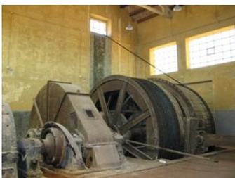
**The Winch Room** - the winding engine was used to move the cages up and down the shaft in order to transport the miners and the wagons.
